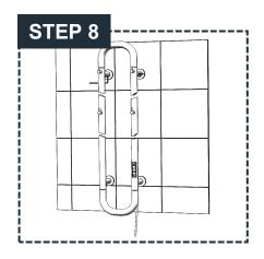
**STEP 8:** Use the Allen wrench to install the hex screws into the holes of all the tubes to complete the installation.
