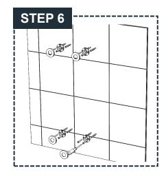
**STEP 6:** Insert the long screws through the mounting seats and then secure them into the plastic wall anchors with a electric drill. Place the decorative caps onto the mounting seats and tighten them.
