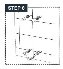
**STEP 6:** Insert the long screws through the mounting seats and then secure them into the plastic wall anchors with a electric drill. Place the decorative caps onto the mounting seats and tighten them.
